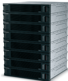
The Lenovo Storage S3200 controller unit with seven E1024 expansion units delivers a total of 192 drives.
